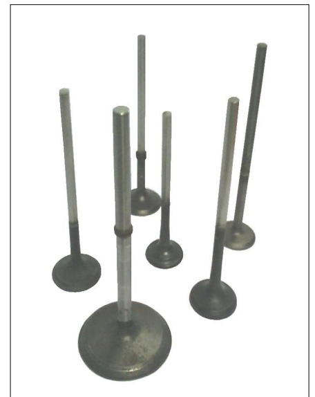
Typical Engine Valves after welding Head to Pin
