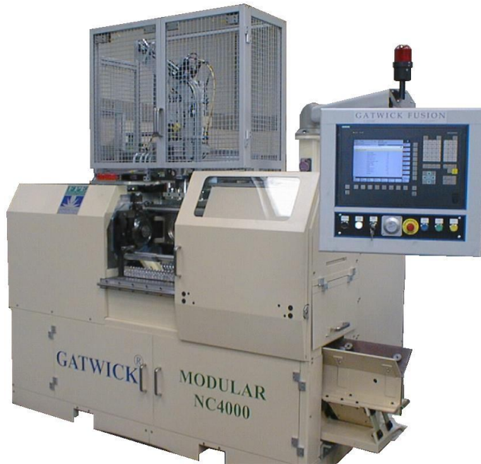
NC4000 with automatic part feeding of valve heads and stems
